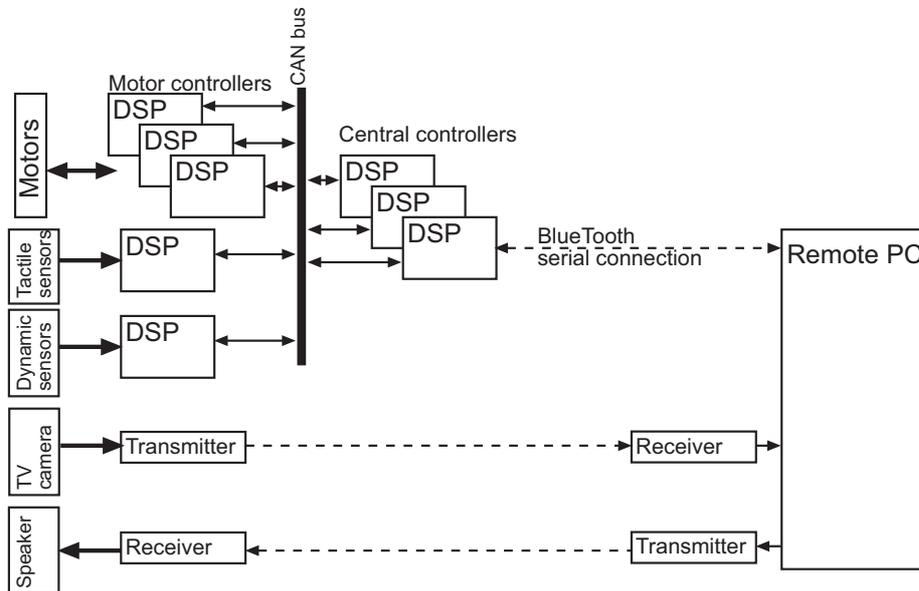
Fig. 3. Block diagram of ARNE-02 control system
